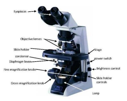
Diagram of a typical bright-field compound microscope. Though various styles exist, all compound microscope have the same basic components and they are labeled in the picture above.
