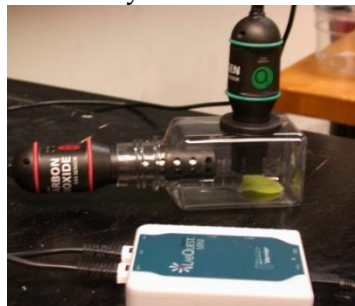
Respiration chamber, sensors and hub.
