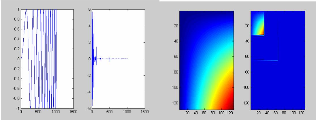
Below, figure 1 shows the original 2D signal with a perturbation (square dot), and the same signal with an added noise (30% of the signal amplitude). Figure 4 shows the original signal, the Fourier and wavelet transform of the same signal with added noise. The perturbation (square dot) is not seen in the Fourier transform but yes in the wavelet transform.
