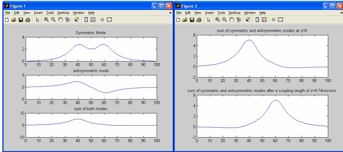
After a coupling length of  $z=4.74$  microns, the sum mode is coupled into the other waveguide as seen in the figure above.
