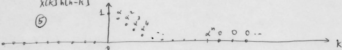
So:  $\left\{ \begin{array}{l} n > 0 \\ \alpha < 1 \end{array} \right\} y[n] = \sum_{k=-\infty}^{\infty} x[k] h[n-k] = \sum_{k=0}^n \alpha^k : \text{sum of a geometric series}$
