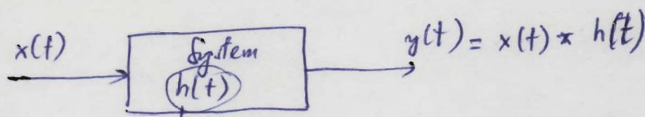
Impulse response : if the output to the  $\delta(t)$  input:
