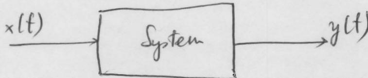
$$y(t) = 2x(t) - x^2(t+1) \rightarrow \text{This is the "input-output" equation.}$$
