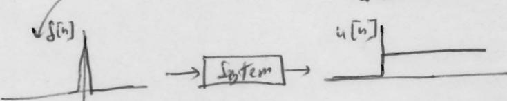
Switch: When you turn the switch @  $t=0$ ; i.e. the  $\delta[n]$  input, the light turns on and stays on; i.e.; the step function.
