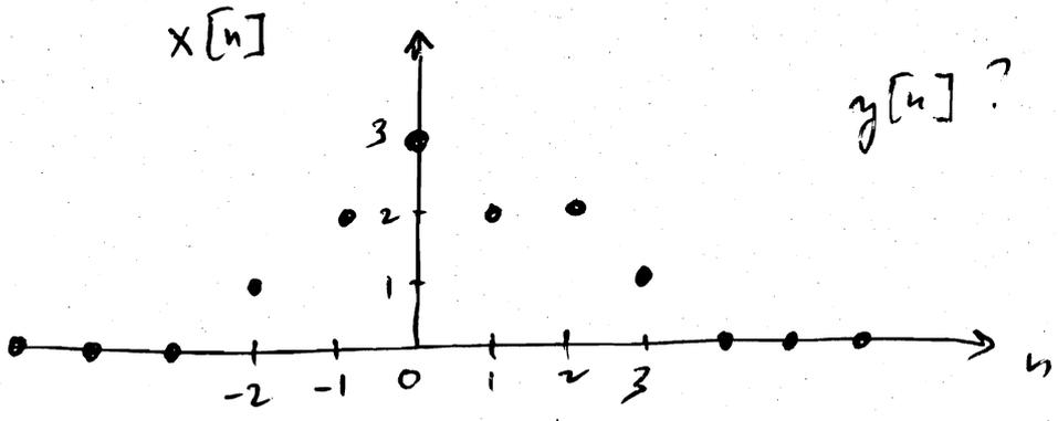
System initially at rest :  $y[n] = 0$  when  $x[n] = 0$
