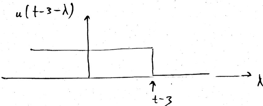
$$y(t) = 2 \int_0^{t-1} d\lambda \sin \pi \lambda - 2 \int_0^{t-3} d\lambda \sin \pi \lambda - 2 \int_2^{t-1} d\lambda \sin \pi \lambda + 2 \int_2^{t-3} d\lambda \sin \pi \lambda$$
