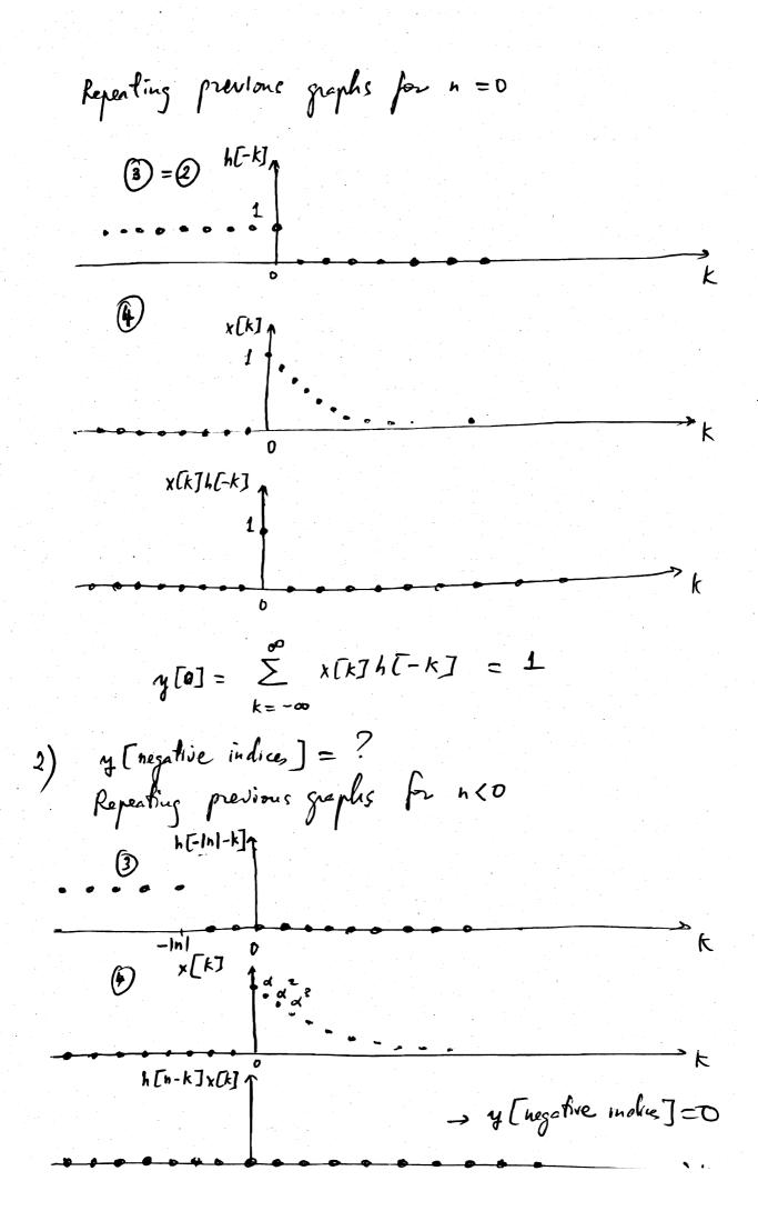
$$\frac{x[n] = \alpha^{n}u[n]}{h[n] = u[n]} \frac{y[n]}{y[n]} \begin{pmatrix} D & n < b \\ 1 & n = 0 \\ \frac{1-\alpha^{n+1}}{1-\alpha} u[n] \end{pmatrix} = \frac{1-\alpha}{1-\alpha} u[n]$$
