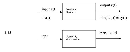
Input/output difference equation for  $S_1$  is  $y_1[n] = 2x_1[n] + 4x_1[n-1]$
