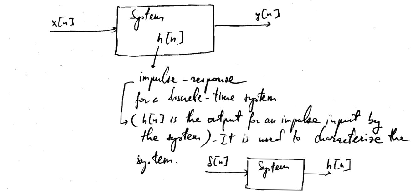
$$y[n] = x[n] * h[n] \quad (y[n] \text{ is } x[n] \text{ convolution with } h[n])$$
