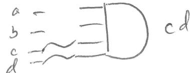
fuses on a & b are blown  $\rightarrow$  open connections for AND gates are 1's; open connections OR gates are 0's.
