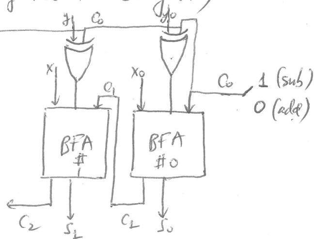
Note: this works in sequence: need to wait until the carry-out is produced before the next add/sub → "ripple effect".
