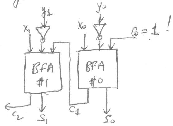
We can combine these into one combination that allows performing addition or subtraction by the same two  $n$ -digit binary numbers via a switch (of the 1<sup>st</sup> carry in)
