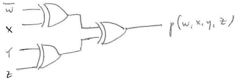
$\left\{ \begin{array}{l} 3 \text{ XOR's} \rightarrow 3 \text{ 7486 IC's} \\ 8 \text{ four-input AND's} \end{array} \right.$  versus
