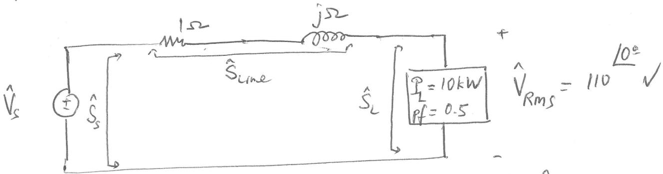
Calculate  $\hat{V}_s$  so the circuit can deliver the specified load.
