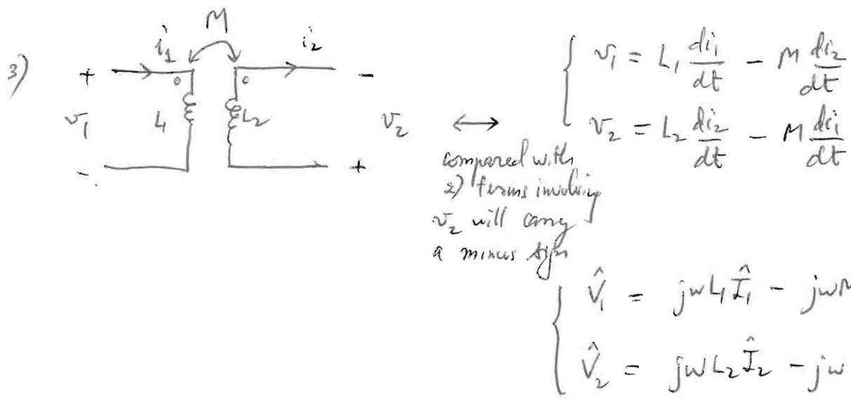
Example: AC Analysis of circuits with more than one inductor:
