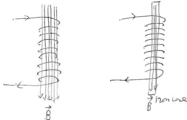
can set a fixed cross-section for the magnetic flux by using an iron core
