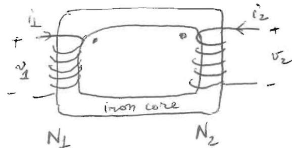
→ Faraday's Law: voltage  $v_1$  comes from a change of magnetic flux through solenoid #1:  $N_1 \frac{d\phi_1}{dt}$
