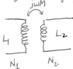
→ Two solenoids with different inductances  $L_1$  &  $L_2$  (different cross section, numbers of turns, etc.)
