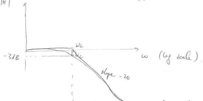
This RC arrangement passes components with  $\omega < \omega_c$ , and blocks components with  $\omega > \omega_c$ , i.e. it is a low-pass filter.
