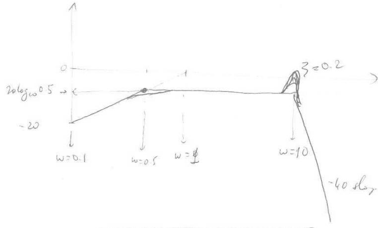
Phase Bode Plot:  $\hat{H}(j\omega) = \frac{0.5j\omega}{(1 + j\frac{\omega}{0.5})(1 + j\frac{\omega}{10})^2 + (j\frac{\omega}{10})^2}$
