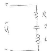
$$\begin{aligned}\hat{Z}(j\omega) &= R + j\omega L + \frac{1}{j\omega C} \\ &= R + j\left(\omega L - \frac{1}{\omega C}\right) \\ \omega_0 L &= \frac{1}{\omega_0 C} \rightarrow \omega_0 = \frac{1}{\sqrt{LC}}\end{aligned}$$
