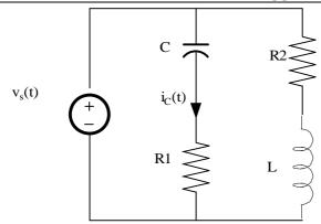
AT RESONANCE  $V_S(t)$  AND  $I_S(t)$  ARE IN PHASE. SO, THE IMPEDANCE SEEN BY THE SOURCE,  $Z_S$ , IS PURELY RESISTIVE.
