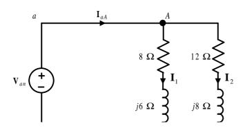
$$I_1 = \frac{120\angle 20^\circ}{8+j6} = 12\angle -16.87^\circ \text{ A rms}$$
