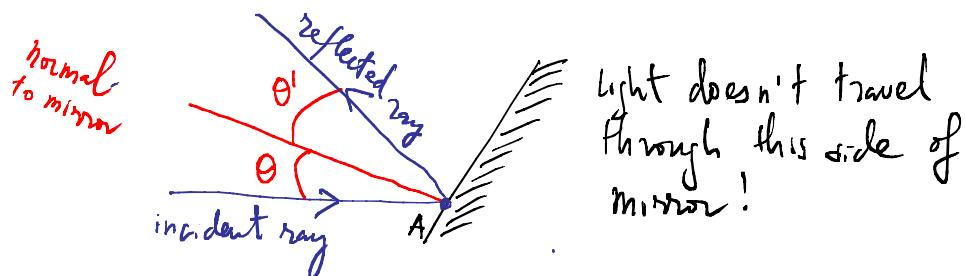
→ Normal direction: perpendicular to mirror @ incident point A
