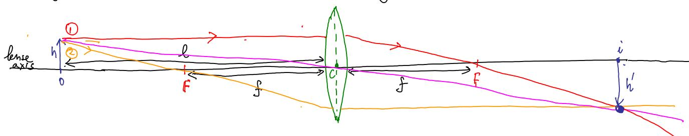
Ray tracing  $\left\{ \begin{array}{l} \text{(1) Incident ray } \parallel \text{ axis emerges from F the other side of lens} \\ \text{(2) Incident ray from left F, emerges } \parallel \text{ axis the other side of lens} \\ \text{(3) Incident ray thru center of lens C, keeps its direction.} \end{array} \right.$
