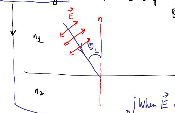
When  $\vec{E}$  oscillates  $\perp$  to incident ray and in plane with page as shown and if  $\theta_i = \theta_p$  then there is no reflection at the boundary, all energy travels in second medium  $n_2$
