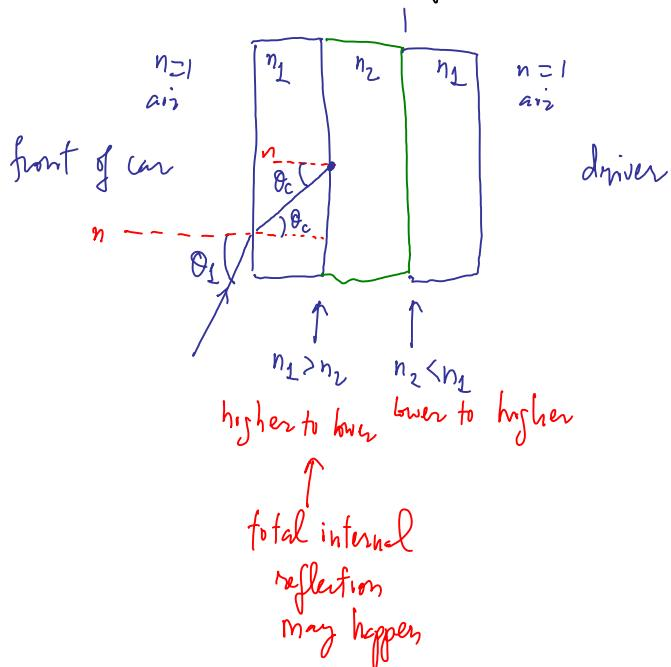
We want to calculate what incident angle  $\theta_1$  would refract into a ray that hits the 2nd boundary @ critical angle  $\theta_c$  which leads to total internal reflection (reduces visibility)
