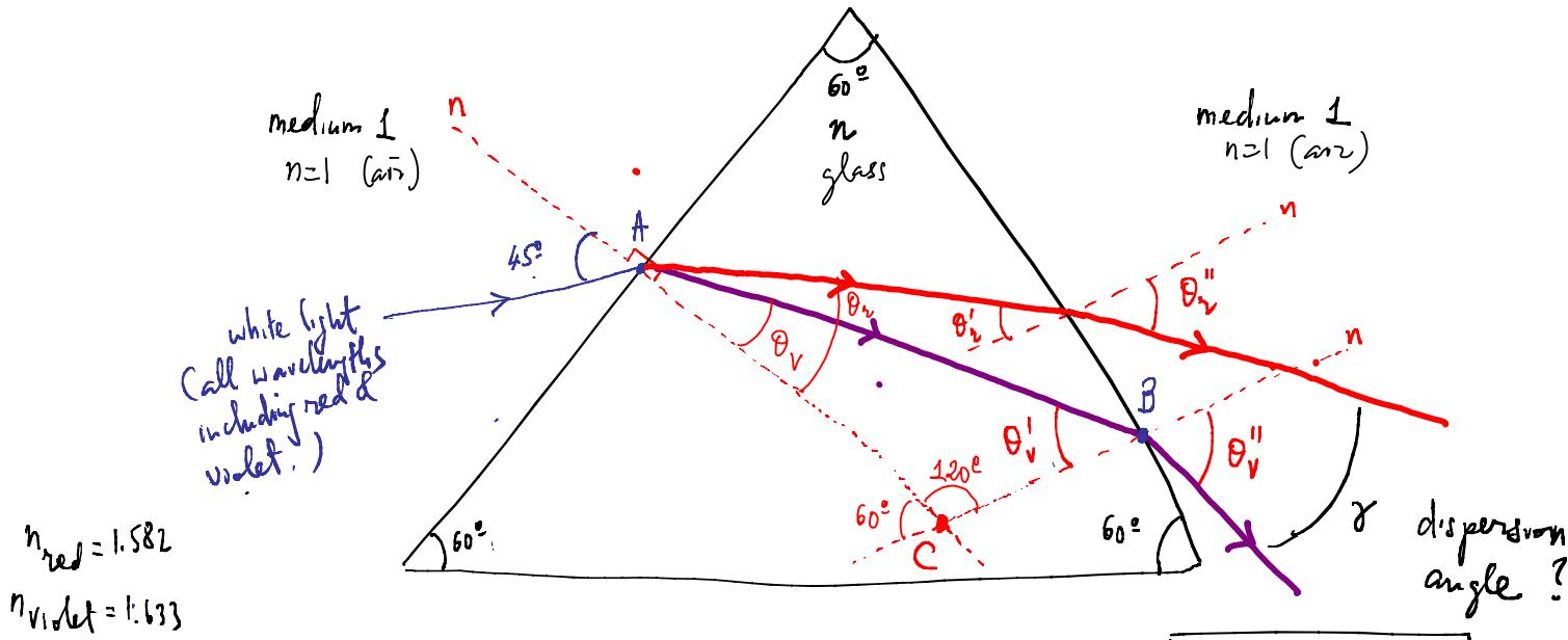
White light beam incident of left side of prism is spread out after refractions by prism  $\rightarrow$  determine dispersion angle  $\gamma$ .
