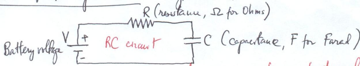
Simpliest circuit to charge a capacitor or to store electrostatic potential energy
