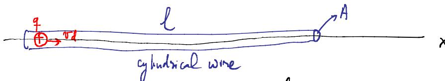
U<sub>d</sub>: drift velocity: average velocity along wire axis (normally small as it is an average over a random distribution of actual velocities)
