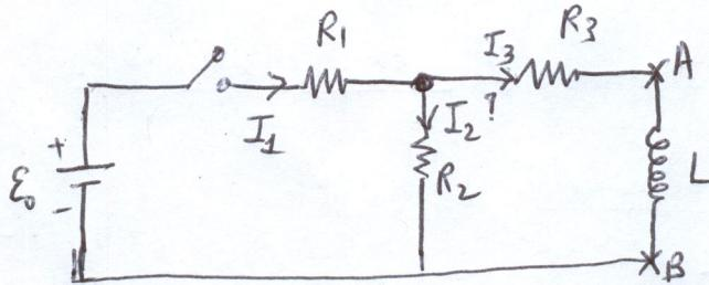
$$\begin{aligned} E_0 &= 12V \\ R_1 &= 4\Omega; R_2 = 8\Omega; R_3 = 2\Omega \\ L &= 2H \end{aligned}$$
