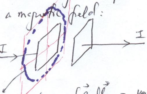
$$\text{Amperian loop: } \oint \vec{B} \cdot d\vec{l} = \mu_0 I_{\text{Enclosed}}$$
