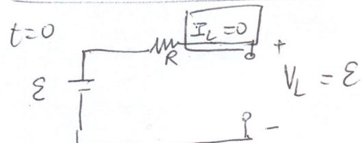
→ As circuit is closed,  $I_L$  was 0, stays at 0,  $I_L$  does not change instantaneously
