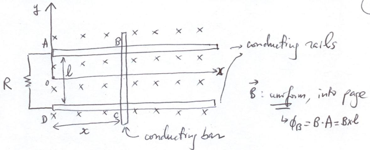
Magnetic flux through ABCD depends on position  $x$  of conducting bar
