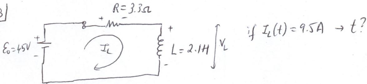
Inductor is an inertia to current  $I_L$ : before switch was closed  $I_L = 0$ ,  $I_L(0) = 0$  then it starts to build up, till it gets to the max. value when  $V_L = 0$  (short circuit when  $t \rightarrow \infty$ )
