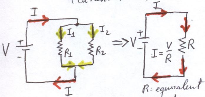
1)  $I = I_1 + I_2$  Current division for  $R_1$  &  $R_2$
