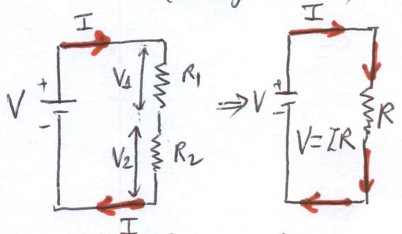
1)  $V = V_1 + V_2$  Voltage division
