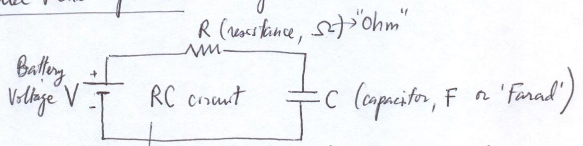
↳ Simplest circuit to charge the capacitor or to store electrostatic energy
