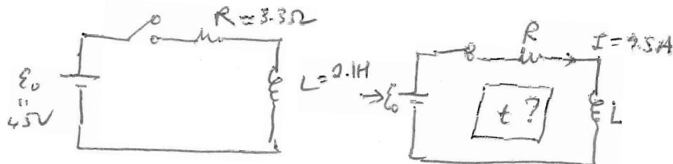
$L$  is an inductor to current  $I$ : when switch is closed the current is still 0: current will build up from  $0 \rightarrow \text{max.}$
