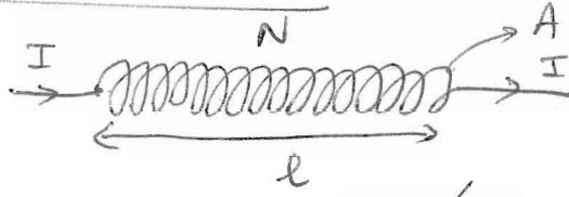
$$\left\{ \begin{array}{l} B_{\text{solenoid}} = \mu_0 n I \\ n = \frac{N}{l} \end{array} \right.$$
