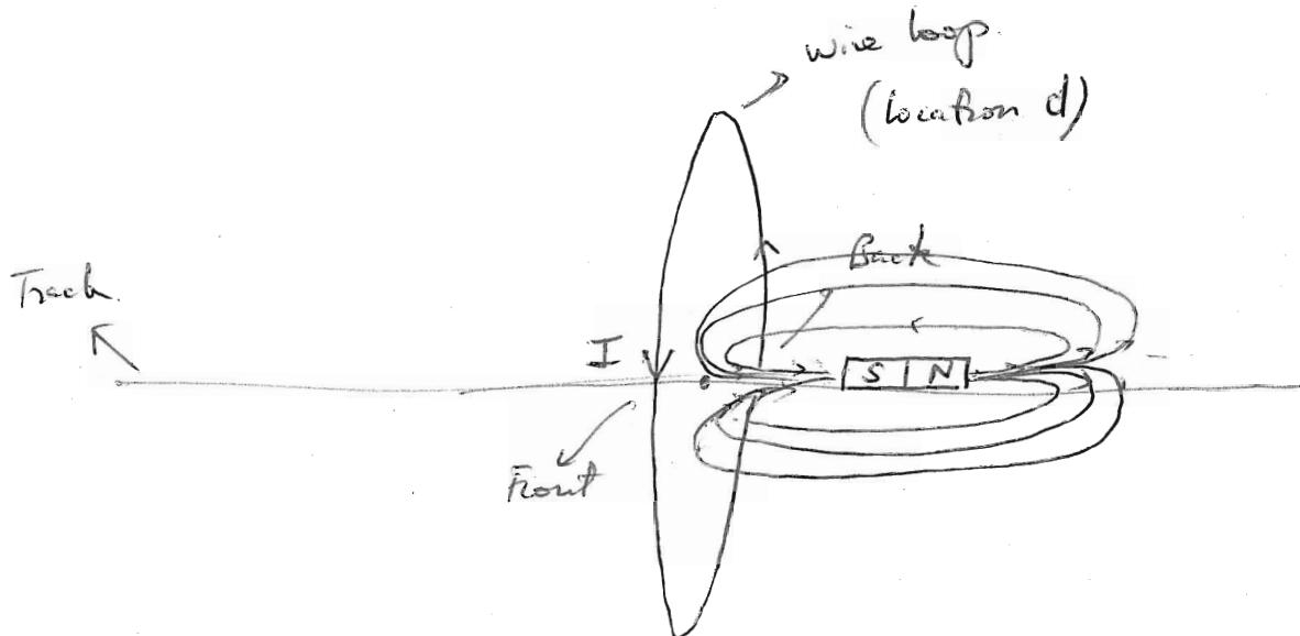
3) As magnet continues sliding beyond loop: as magnet is leaving the loop: there is a decreased magnetic flux through the surface area enclosed by wire loop  $\rightarrow$  induced voltage will create an induced current such that it will create an induced magnetic field pointing in  $+z$  (same as original field by magnet) so induced current now is downward in the front of loop or CCW if viewed from right of loop.
