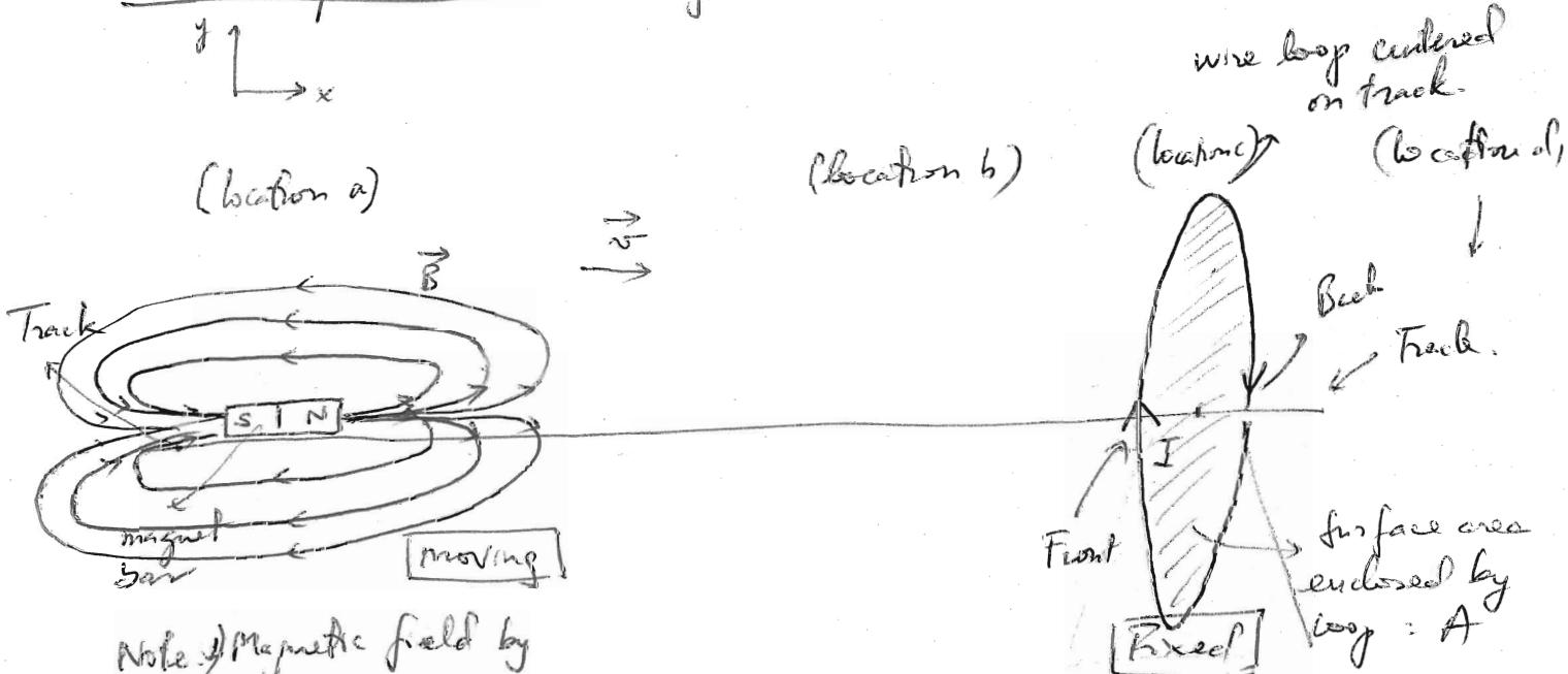
Note: Magnetic field by magnet is stronger closer to the poles, pointing in +i along track.
