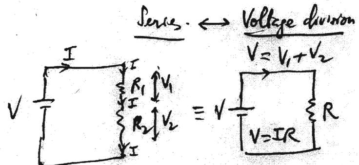
$R_{eq}$  is the equivalent resistor for  $R_1$  &  $R_2$ :
