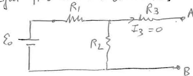
$$= E_0 \left\{ \begin{array}{l} R_1 \\ R_2 \end{array} \right\} \frac{I_2 = \frac{E_0}{R_1 + R_2}}{R_1 + R_2} = \frac{12}{4+8} = 1A$$
