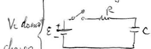
$V_c$  does not change  $t=\infty$  long after switch was closed  $\rightarrow$  open circuit across  $L$  as switch is closed  $I_c = 0$   $I_c = \frac{E}{R} e^{-\frac{t}{RC}}$
