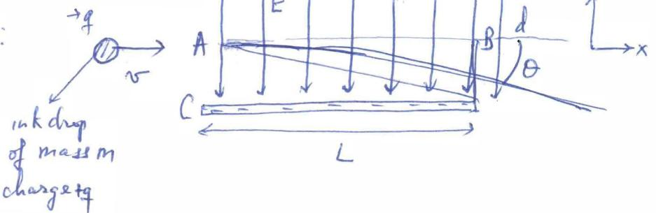
Ink drop while crossing field region, feels a downward force  $\rightarrow$  a downward acceleration  $\rightarrow a_y = \frac{F}{m} = \frac{qE}{m}$   $\rightarrow$  constant downward acceleration!
