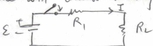
As circuit is closed :  $V_{R_1}$  &  $V_{R_2}$  as well as I come up to their final values instantaneous.
