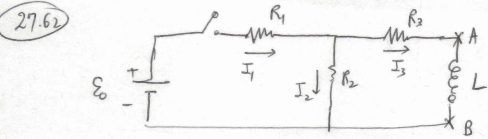
$$\begin{cases} E_0 = 12V \\ R_1 = 4\Omega \\ R_2 = 8\Omega \\ R_3 = 2\Omega \\ L = 2H \end{cases}$$
