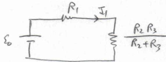
(Parallel combination b/w  $R_2$  &  $R_3$ )
