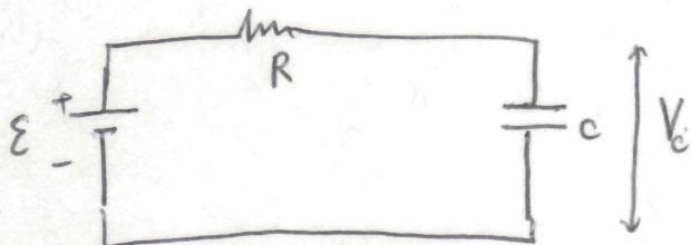
Used to charge a capacitor
