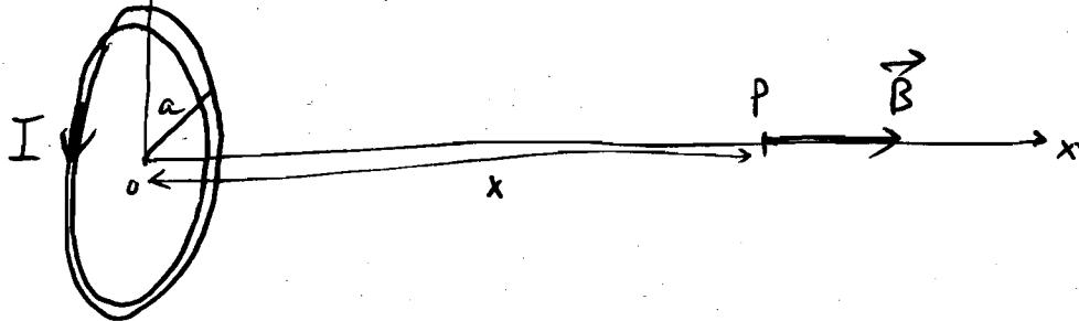
$$\vec{B} = B(x)\hat{i}; \quad B(x) = \frac{\mu_0}{2} \frac{Ia^2}{(x^2 + a^2)^{3/2}} \quad (\text{T for Tesla, S.I.})$$
