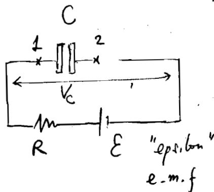
At  $[t=0]$  we connect the uncharged capacitor:  $Q=0$ ,  $V_C=0$ : thus is like: a shortcircuit across  $1 \& 2$  (like a wire is connecting  $1 \& 2$ )
