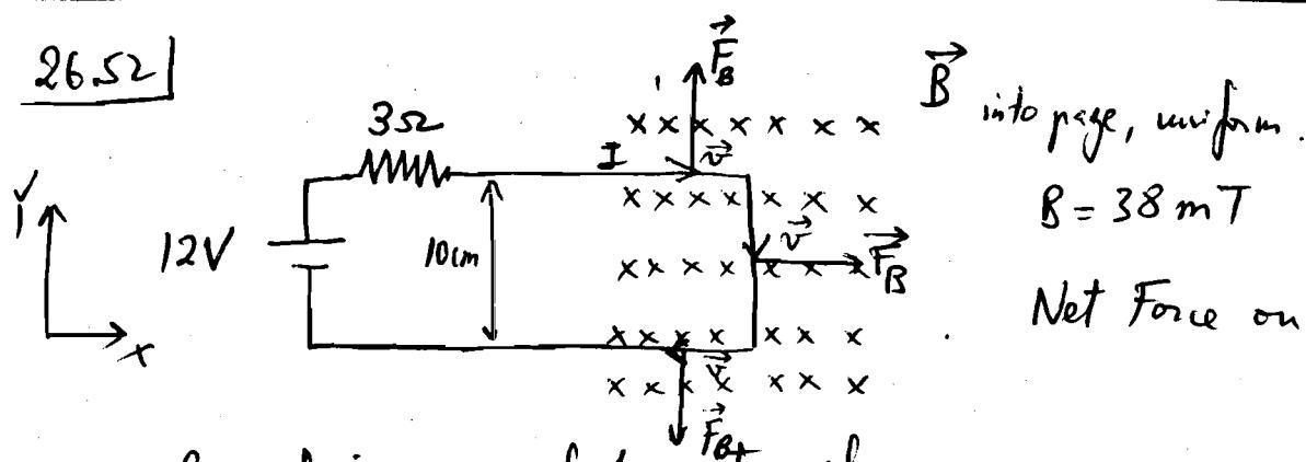
Current is composed of positive charges moving along the loop. The top & bottom force are equal & opposite b/c = same  $v$  &  $B$  (or same current) & same  $B$  b/c it's uniform. Net force is due to  $\vec{F}_B$  on vertical side immersed in the field region:
