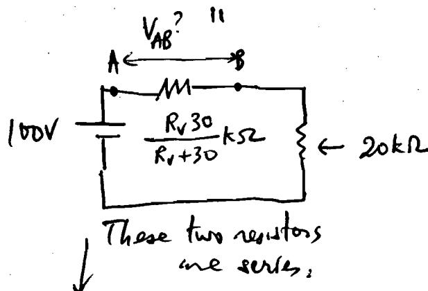
$$\begin{aligned} & \text{(parallel of } 40 \text{ k}\Omega \text{ & } 20 \text{ k}\Omega) \\ & \frac{40 \times 20}{40 + 20} \text{ k}\Omega = \frac{1600}{60} \text{ k}\Omega \\ & = 20 \text{ k}\Omega \end{aligned}$$
