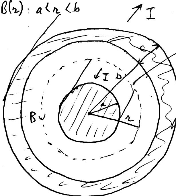
→ Amperian loop : can factor  $B$  out of the left hand side integral:
