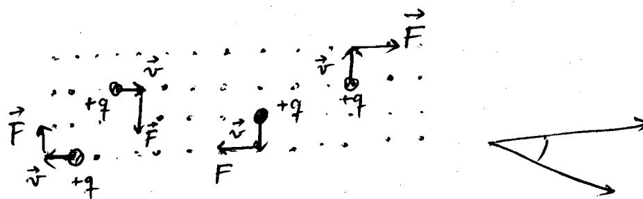
So: the trajectory of a charged particle in a magnetic field is circular, since  $\vec{F}_B$  is always perpendicular to the direction of motion, being the agent that provides the radial acceleration:
