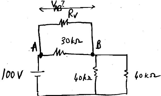
$$R_V = \begin{cases} a) & 50 \text{ k}\Omega \\ b) & 250 \text{ k}\Omega \\ c) & 10^4 \Omega = 10000 \text{ k}\Omega \end{cases}$$
