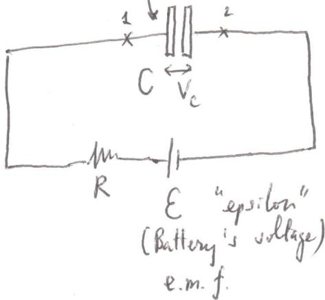
$t=0$  we connect the uncharged capacitor
