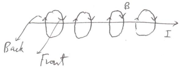
Example: Magnetic field produced by a loop of current =
