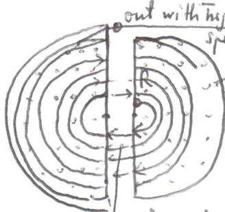
$\vec{B}$  uniform, out of page to keep charged particle in circular motion within the two half-circles
