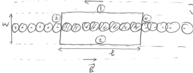
$$\oint \vec{B} \cdot d\vec{l} = \underbrace{B \cdot l}_{(1)} + \underbrace{Bl}_{(2)} + \underbrace{0w}_{(3)} + \underbrace{0w}_{(4)}$$
