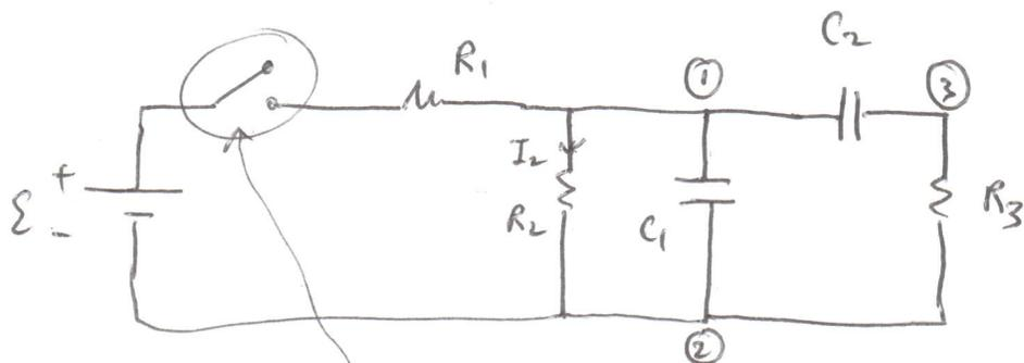
What  $I_2$   $\left\{ \begin{array}{l} \text{a) switch is just closed} \rightarrow (t=0) \\ \text{b) long after switch is closed} \rightarrow (t=\infty) \end{array} \right.$
