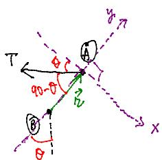
Step 3: Equations  $\left\{ \begin{array}{l} 1) Mg_{\text{wind}} - T \cos \theta - \mu N = 0 \\ 2) N - Mg_{\text{wind}} - T \sin \theta = 0 \\ 3) r_{BA} T \cos \theta = r_{BC} \mu N \end{array} \right\}$  static equilibrium of the pole
