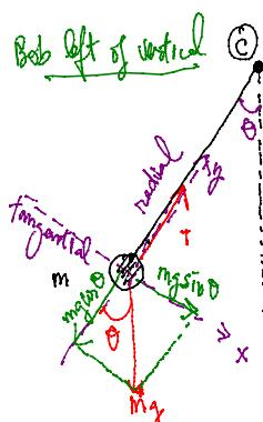
$$\begin{aligned} F_{\text{ref},x} &= mg \sin \theta = m a & a = +g \sin \theta \\ F_{\text{ref},y} &= T - mg \cos \theta = 0 \end{aligned}$$
