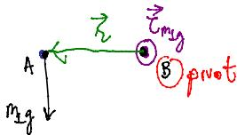
$$\vec{\tau}_{mg} = \vec{r} \times (m g \hat{k}) = r_{mg} \underbrace{(\hat{j} \times (-\hat{k}))}_{\text{RHR: out of page } \hat{i}} = r_{BA} m g \hat{i}$$
