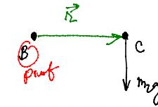
$$\begin{aligned} \vec{\tau}_{mg} &= \vec{r} \times (-m g \hat{k}) \\ &= r_{BC} m g (\hat{j} \times (-\hat{k})) \\ &\quad \cdot \text{RHR: into page } (-\hat{i}) \\ &= -r_{BC} m g \hat{i} \end{aligned}$$
