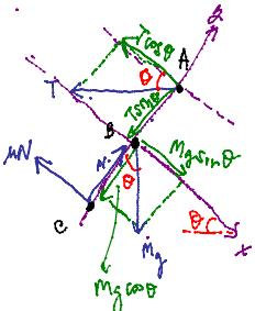
$$i) \vec{F}_{net} = 0 \quad \begin{cases} F_{net,x} = 0 = Mg \sin \theta - T \cos \theta - \mu N = 0 \quad (1) \\ F_{net,y} = 0 = N - Mg \cos \theta - T \sin \theta = 0 \quad (2) \end{cases}$$
