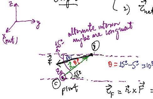
$$\vec{r}_{\text{pivot}} = \vec{r} \times \vec{F} = r_{CD} F \sin 10^\circ \hat{i} \quad \text{RHR}$$
