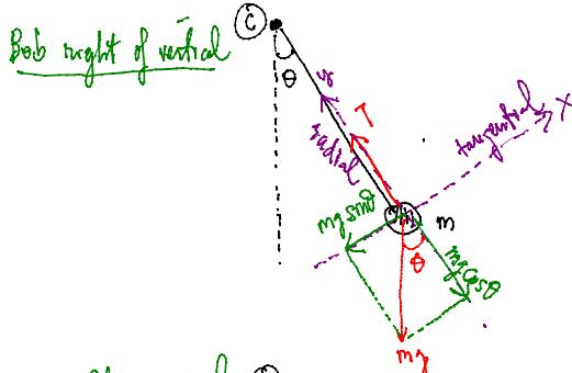
$$\begin{aligned} F_{\text{ref},x} &= -mg \sin \theta = m a & a = -g \sin \theta \\ F_{\text{ref},y} &= T - mg \cos \theta = 0 \end{aligned}$$
