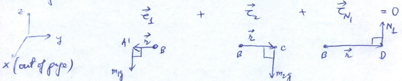
$$m_1 g r_{BA1} \underset{\text{RHR}}{+} m_2 g r_{BC} \underset{\text{RHR}}{+} N_1 r_{BD} (i) = 0$$
