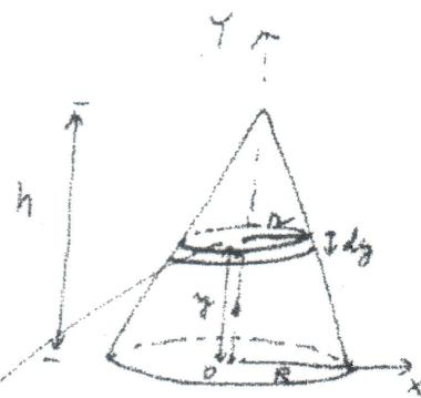
infinitesimal disk of thickness  $dy$  & mass  $dm$ ,
