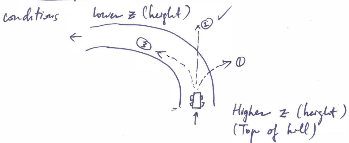
Vehicle would follow path ② : the agent or force that would normally pull the vehicle toward the center of curvature is absent. That is the friction force b/w tires & road is absent.
