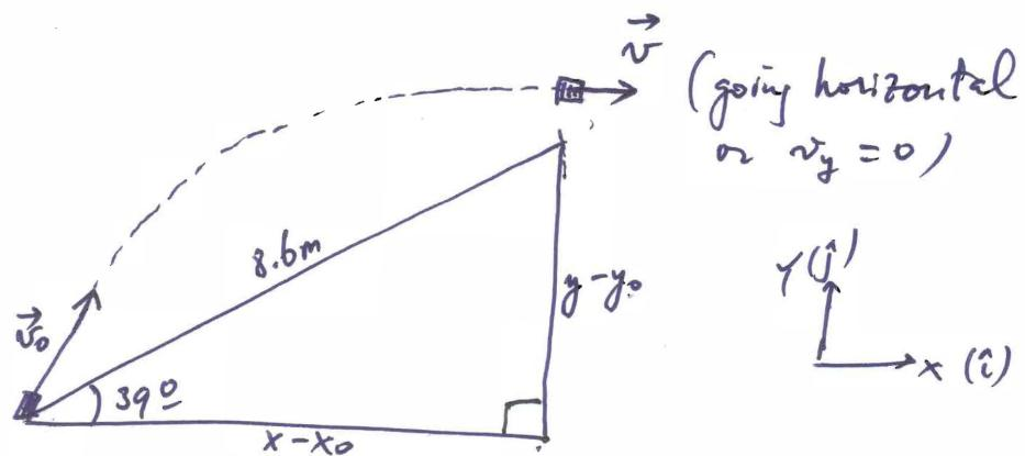
Chocolate bar  $\left\{ \begin{array}{l} \vec{v}_0 ? \\ \vec{v} = v_x \hat{i} \end{array} \right\}$  It follows the 1<sup>st</sup> half of a projectile motion under the effect of gravity  $\Rightarrow \vec{a} = 0\hat{i} - g\hat{j}$
