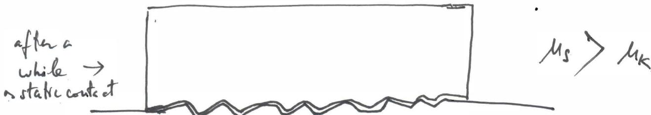
Observation: when you try to push a heavy box, you would apply increasing force until you reach the threshold, (to overcome the static friction  $F_s$ ) then it starts moving fast → this is because you still applying the threshold force while  $F_s$  is reduced to  $F_k$  as the object starts moving, this gives a net force forward → accelerates the object forward
