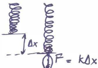
Let's focus on the fish:  $\vec{F}_{\text{net}} = (\vec{F}_{\text{spring}} - \vec{mg})$
