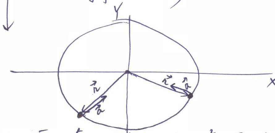
Acceleration is always towards the center of the circular trajectory, since it is keeping the object on the circle
