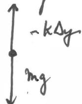
If system is static  $\rightarrow a = 0 \rightarrow F_{\text{net}} = mg - k\Delta y = ma$
