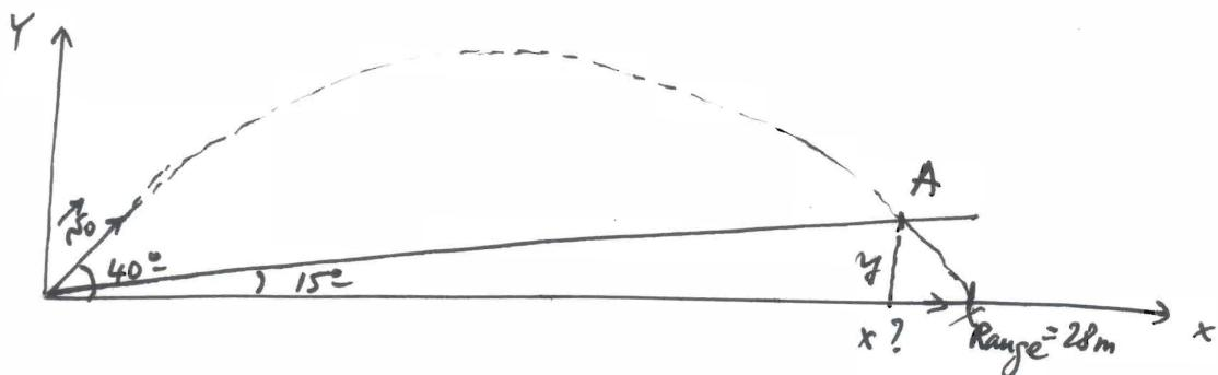
On a slope the range (for same  $\vec{v}_0$ ) will be less since the slope intersects with the parabola (projectile trajectory) at a prior point.
