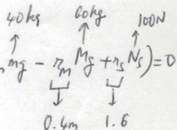
$$r_m = \frac{0.4 \times 60 \times 9.81 - 1.6 \times 100}{40 \times 9.81} = 0.19\text{m} \quad (\text{from pivot})$$
