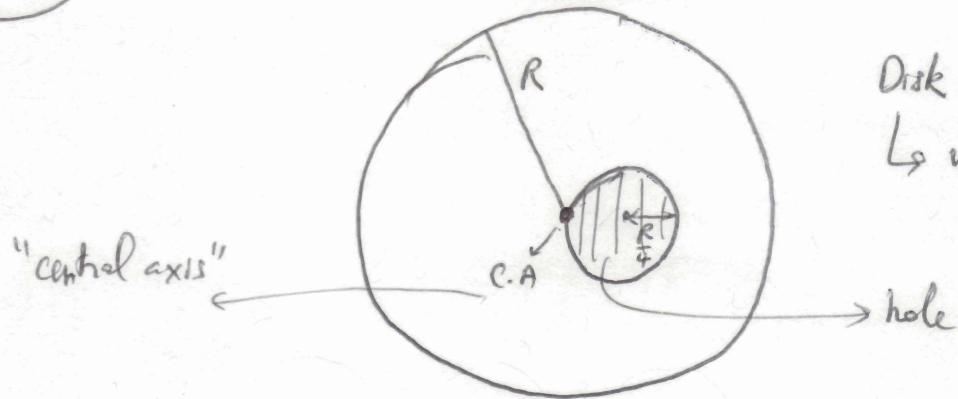
Disk :  $R, M$  $\hookrightarrow$  wrt central axis  $I = \frac{1}{2}MR^2$ Find  $I'$  with the hole; wrt central axis
