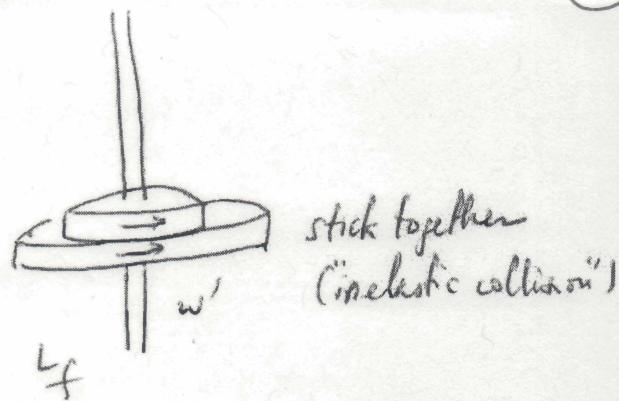
$$\left. \begin{array}{l} R_1 = 2.3 \text{ cm}; m_1 = 0.29 \text{ kg} \\ R_2 = 3.5 \text{ cm}; m_2 = 0.44 \text{ kg} \\ \omega_i = 180 \text{ rpm} \end{array} \right\} \quad \text{Disk}_i = I_{\text{central axis}} = \frac{1}{2} m R^2$$
