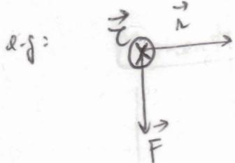
$\vec{r}$  &  $\vec{F}$  in plane of screen:  $\vec{\tau}$  direction (or direction of  $\vec{\tau}$ ) is given by right hand rule
