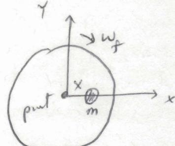
$$\begin{aligned} \text{initial} \\ \vec{L}_i &= I \vec{w}_i + (\vec{r} \times m \vec{v}) \\ &\downarrow \quad \downarrow \\ \text{CW} \rightarrow w_i(-\hat{k}) & \quad \text{only } x\text{-component of } \vec{v} \text{ contributes to cross product} \end{aligned}$$
