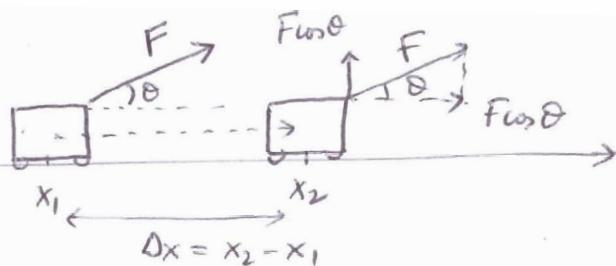
$$\text{Along Y direction } \text{Work} = \underline{F_{\sin\theta}} \cdot \underline{\Delta y} = 0$$
