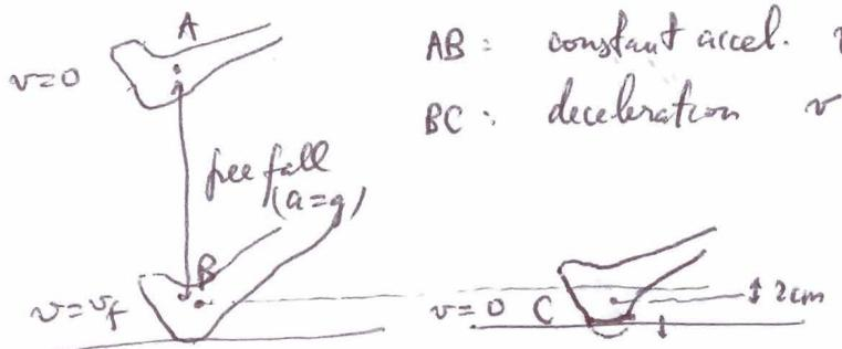
$$AB: \text{constant accel. } v=0 \rightarrow v_f \rightarrow v_f^2 - 0^2 = 2g \Delta x = 2 \times 9.81 \times 0.7$$
