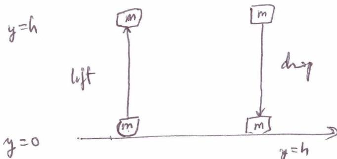
$$\text{lifting} \quad \left\{ \begin{array}{l} \text{Work done by lifter: } \int_{y=0}^{y=h} \vec{F} \cdot d\vec{r} = mg \int_{y=0}^{y=h} dy = mgh \quad (\text{steady upward motion}) \\ \text{Work done by gravity: } -mgh \quad (\text{received work}) \end{array} \right.$$
