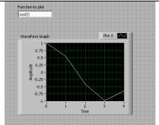
To get a better curve for the cosine function: we need to change the time series: we need to change N, since the graph shows just 5 points (ti, f(ti)) connected with lines. N=41;
