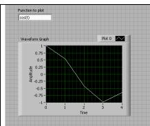
To get a better curve for the cosine function: we need to change the time series: we need to change N, since the graph shows just 5 points (ti, f(ti)) connected with lines. N=41;
