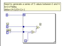
To plot f(t) (vertical axis of our 2D Waveform Graph) versus t (horizontal axis of our Graph), we now need to evaluate f(t) at ti, i.e. obtaining f(ti). Then plot the points (ti, f(ti)) using the Waveform Graph. LabVIEW automatically connect these points with lines. We will enter a function using a String Control in the Front
