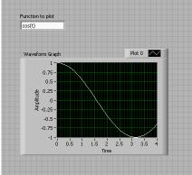
If the number of points is large or the increment  $\Delta$  is small, then the lines are so short that the overall curve looks smooth which resembles the function we are trying to plot.
