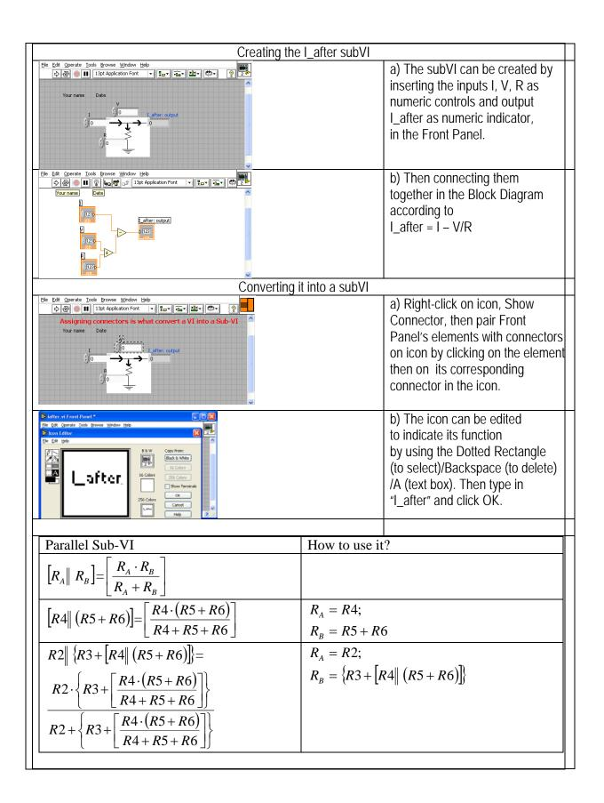
$$I = \frac{V}{R1 + \frac{R2 \cdot \left\{ R3 + \left[ \frac{R4 \cdot (R5 + R6)}{R4 + R5 + R6} \right] \right\}}{R2 + \left\{ R3 + \left[ \frac{R4 \cdot (R5 + R6)}{R4 + R5 + R6} \right] \right\}}} \qquad I = \frac{V}{R1 + R2 \| \left[ R3 + \left[ \frac{R4 \| \left( R5 + R6 \right) \right] \right]}}$$
