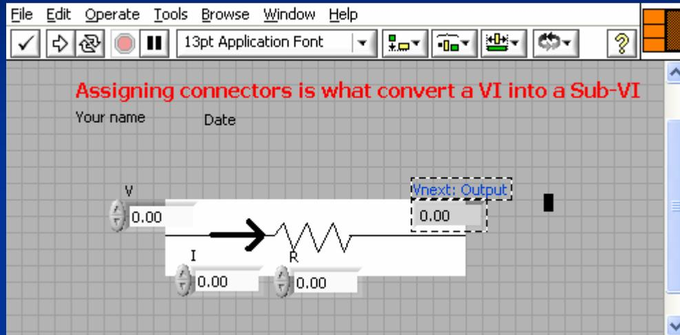
(a) To convert the Vnext VI into a subVI connectors are assigned
