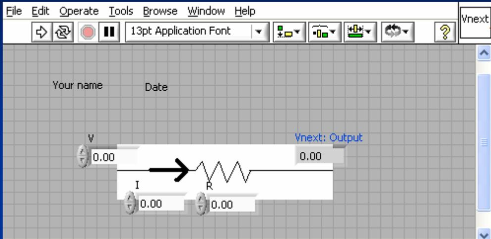
(a) As with the Parallel subVI, we start Creating the VI by placing three numeric Controls labelled as V, I, and R, and One numeric indicator as Vnext
