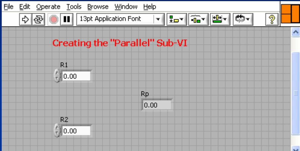
(a) Place two numeric controls labelled As R1 and R2, and one indicator as Rp into the Front Panel
