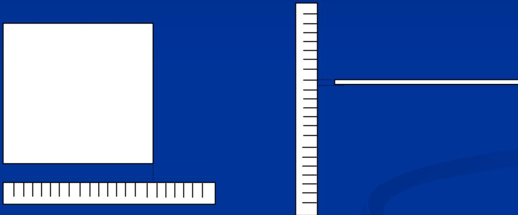
The tolerance for the side dimension X.X is 0.1cm; while for the thickness, it is easier for the eyes to appreciate a half division, i.e. the tolerance for the thickness X.XX is 0.05cm.
