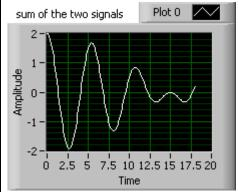
There are two frequency components in this signal, its spectrum will show two peaks
