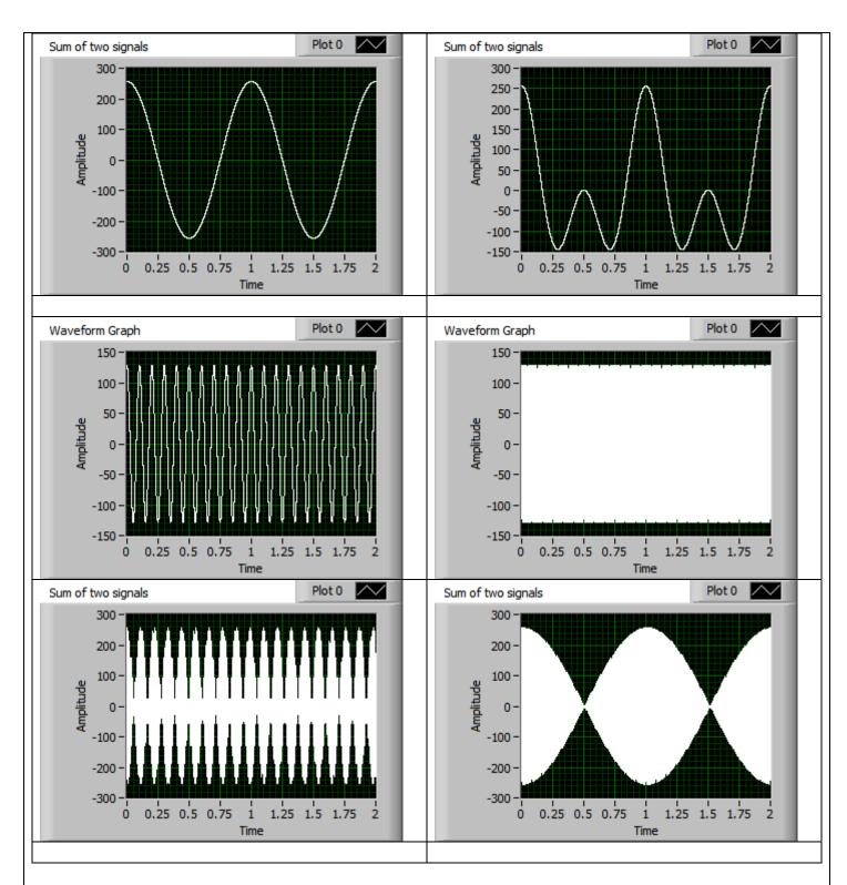
Period T: time separation between consecutive peaks or troughs (time to complete one cycle) Linear frequency f=1/T or number of cycles per second
