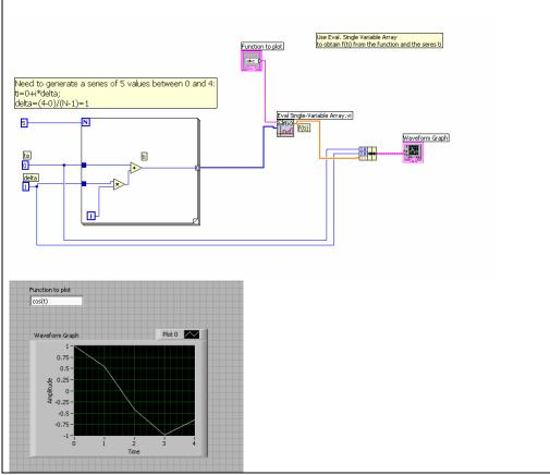
To get a better curve for the cosine function: we need to change the time series: we need to change N, since the graph shows just 5 points (ti, f(ti)) connected with lines. N=41:
