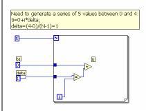
To plot f(t) (vertical axis of our 2D Waveform Graph) versus t (horizontal axis of our Graph), we now need to evaluate f(t) at ti, i.e. obtaining f(ti). Then plot the points (ti, f(ti)) using the Waveform Graph. LabVIEW automatically connect these points with lines. We will enter a function using a String Control in the Front Panel.
