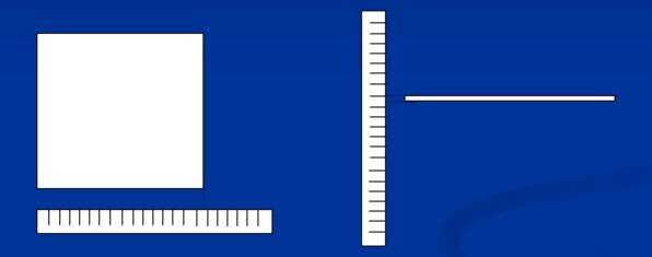
The tolerance for the side dimension X.X is 0.1cm; while for the thickness, it is easier for the eyes to appreciate a half division, i.e. the tolerance for the thickness X.XX is 0.05cm.
