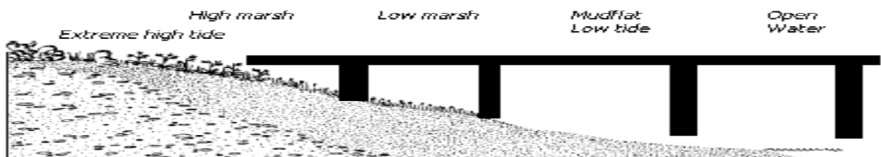
Figure 4: Proposed layout for salt marsh underneath the pier. (Image credit: www.bofep.org with addition by Michael Grealish)
